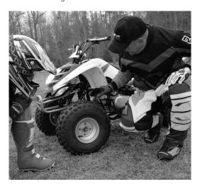
3. Wheels – To avoid loss of control or injury, make sure axle nuts are tight and secured by cotter pins, and make sure wheel nuts are tightened properly. Grasp the tire at the front and the rear and try to rock it on its axle to detect worn-out bearings or loose nuts. There should be no free play or slip as you rock the wheel.
