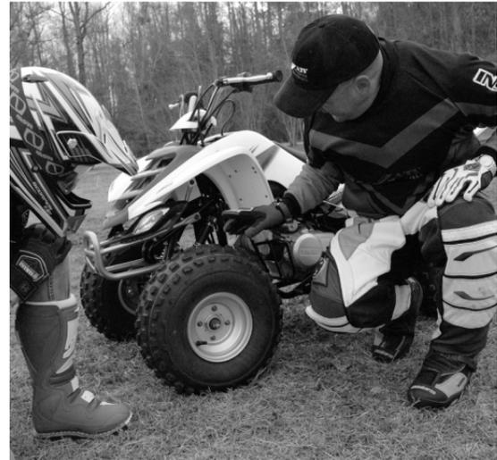
**3. Wheels** – To avoid loss of control or injury, make sure axle nuts are tight and secured by cotter pins, and make sure wheel nuts are tightened properly. Grasp the tire at the front and the rear and try to rock it on its axle to detect worn-out bearings or loose nuts. There should be no free play or slip as you rock the wheel.
